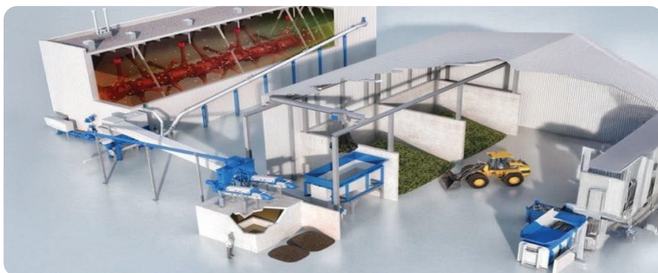
Figure–TTV – Plug Flow Digester 27
