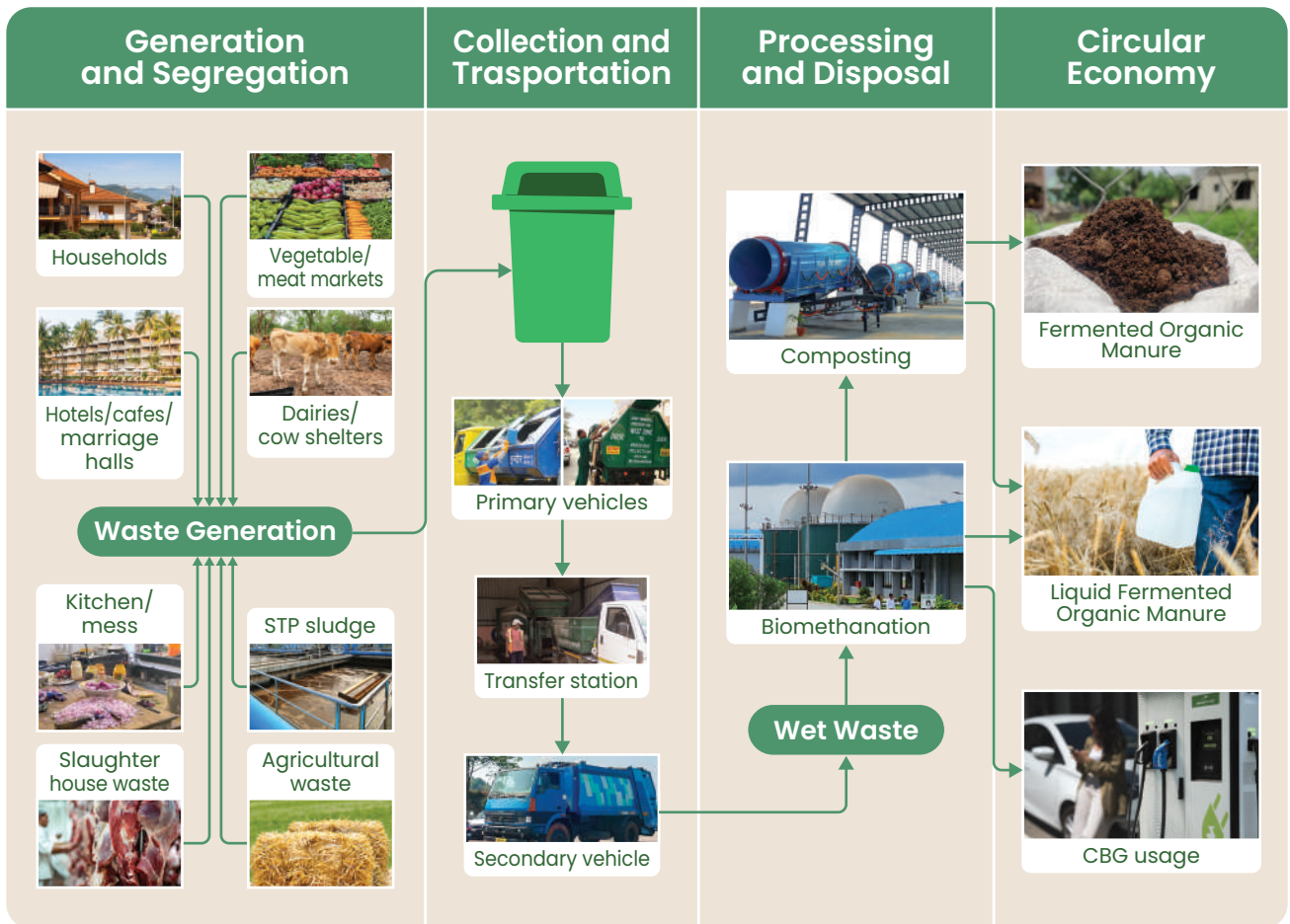
Figure-Value Chain Flowchart of Organic Fraction of MSW from generation to CBG
