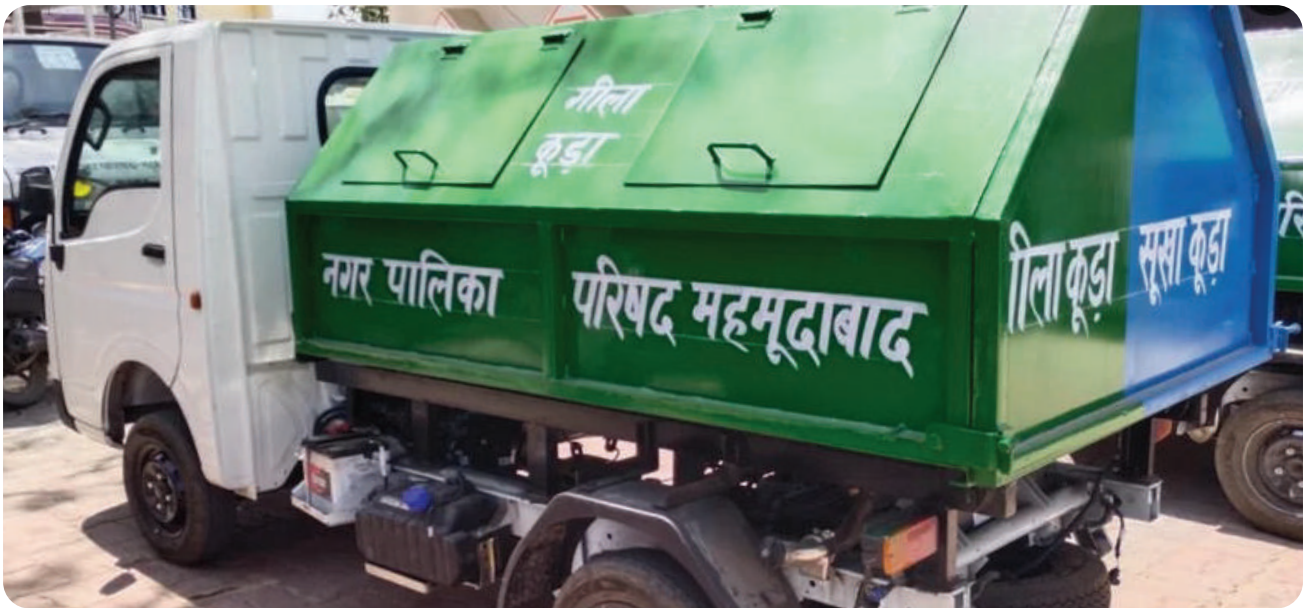
Picture-Partitioned vehicles for transportation of source segregated Wet and Dry fractions
