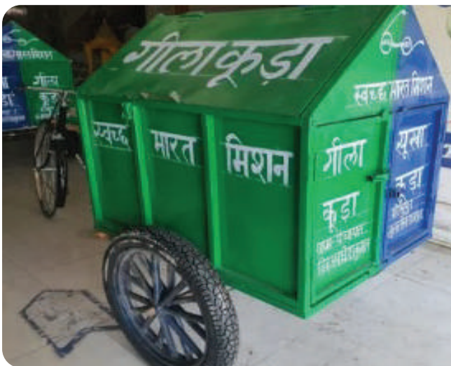
Picture –Partitioned vehicles for transportation of source segregated Wet and Dry fractions
