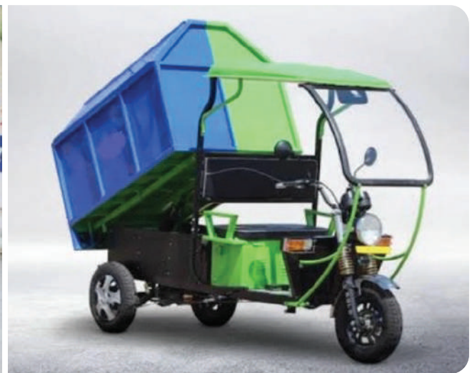
Picture –Partitioned vehicles for transportation of source segregated Wet and Dry fractions
