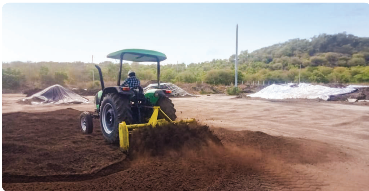
Picture-Drying of FOM at Namakkal CBG project
