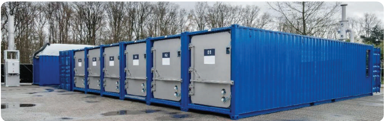
Picture-Representative Image of Transportable Biogas Plant (TBG)
