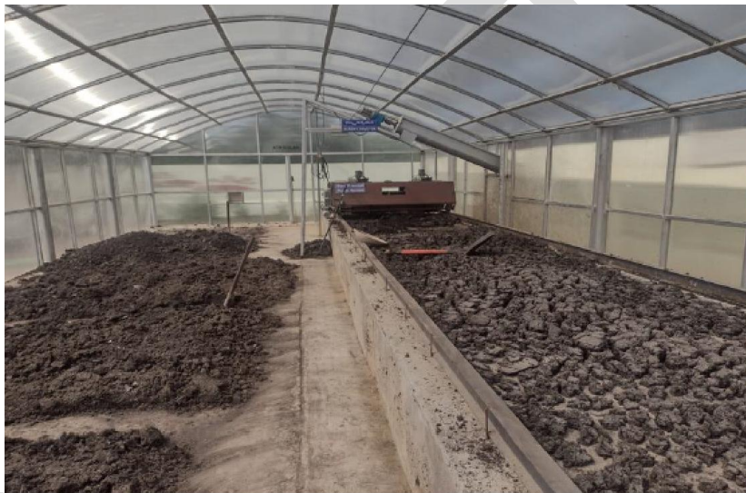
Solar Greenhouse Dryer with Turing machine on SDB
