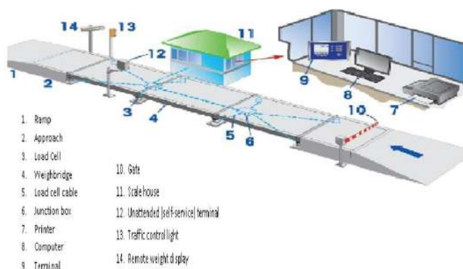
Figure 2: Representative picture for general assembly of Weigh Bridge
