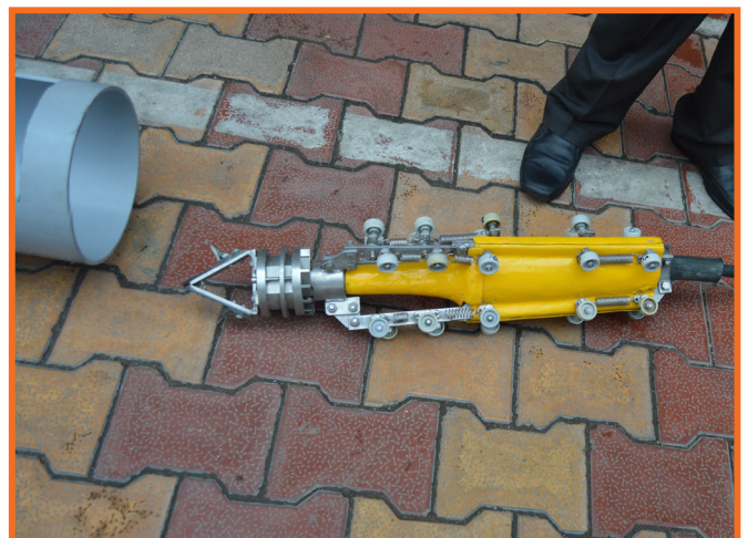
Figure 4 - Sewer Croc (Robotic sewer cutter)
