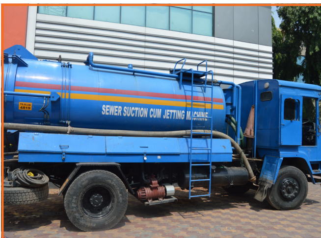
Figure 3 - Hydrovac - Sewer Jetting cum suction
