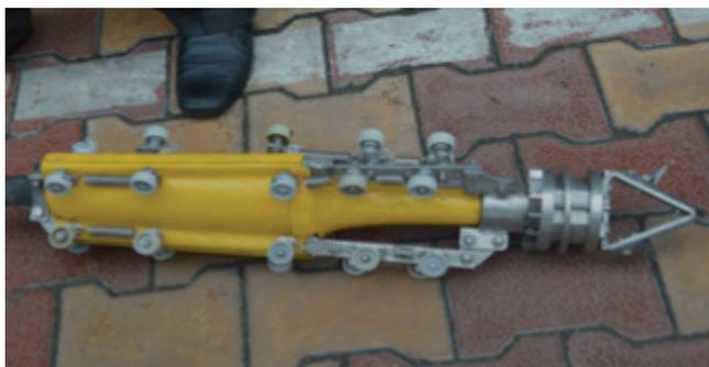
Figure 6 Example of sewer croc
