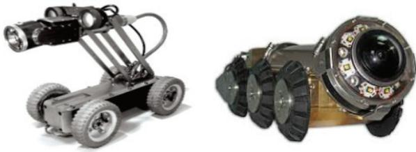
Figure 2 Examples of sewer inspection camera
